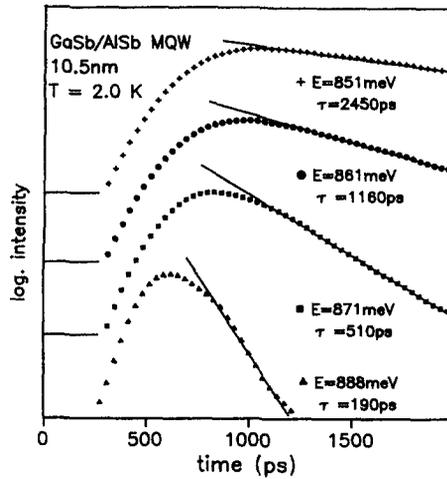
Fig. 1. Decay times for a 10.5nm sample for different energetic positions
