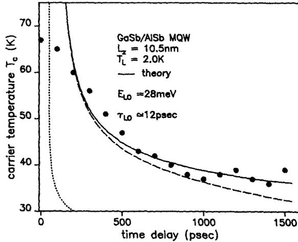
Fig. 3. Carrier cooling curve for a 10.5nm sample; dots: experimental data; curves: theory (see text)
