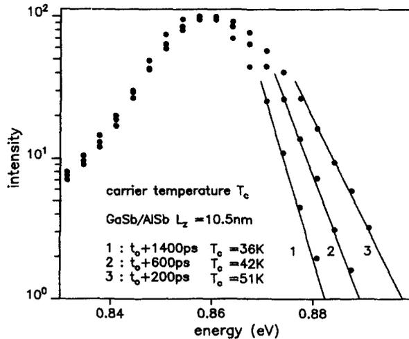
Fig. 2. Determination of the carrier temperature  $T_c$  for different time delays after excitation (at  $t_0$ )
